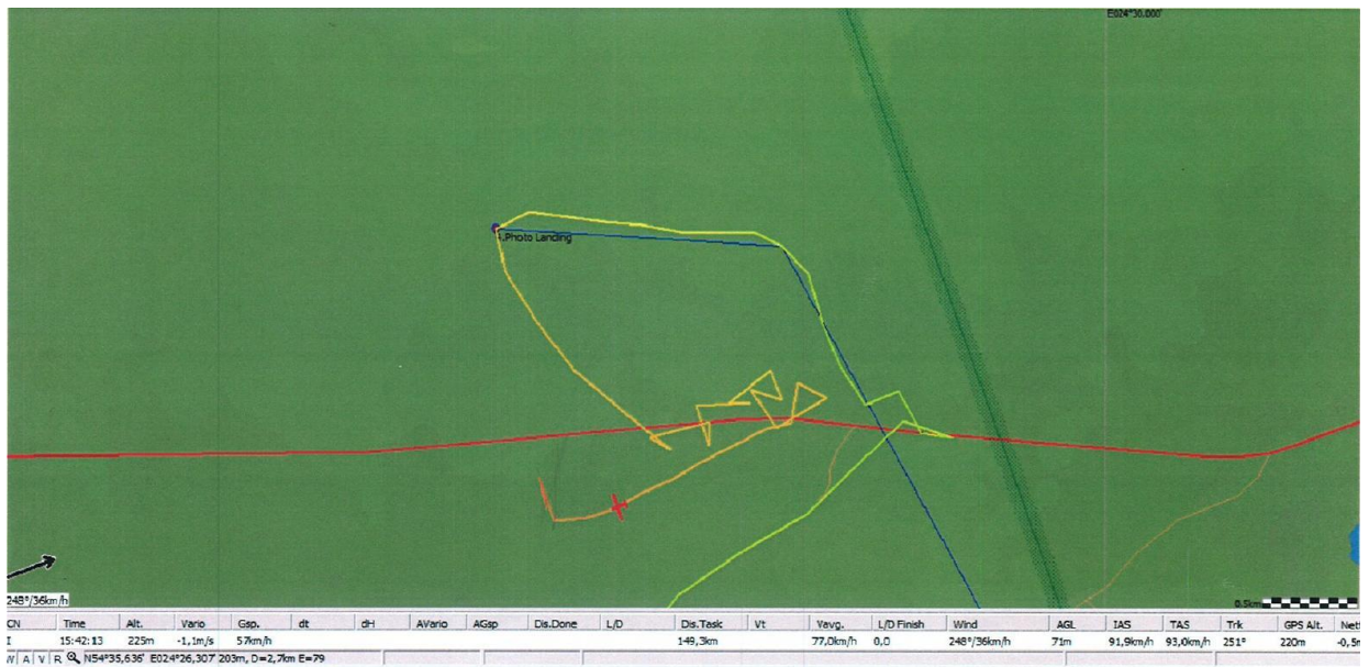
Figure 2. Graphic image of the data on the glider's last flight stage registered by glider GPS data logger.
