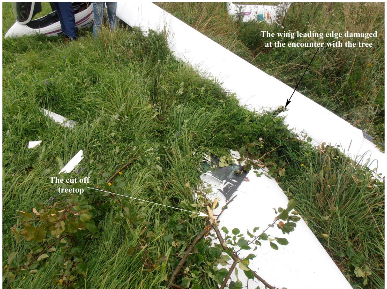
Figure 6. Damaged parts of the wing and remnants of the treetop.
