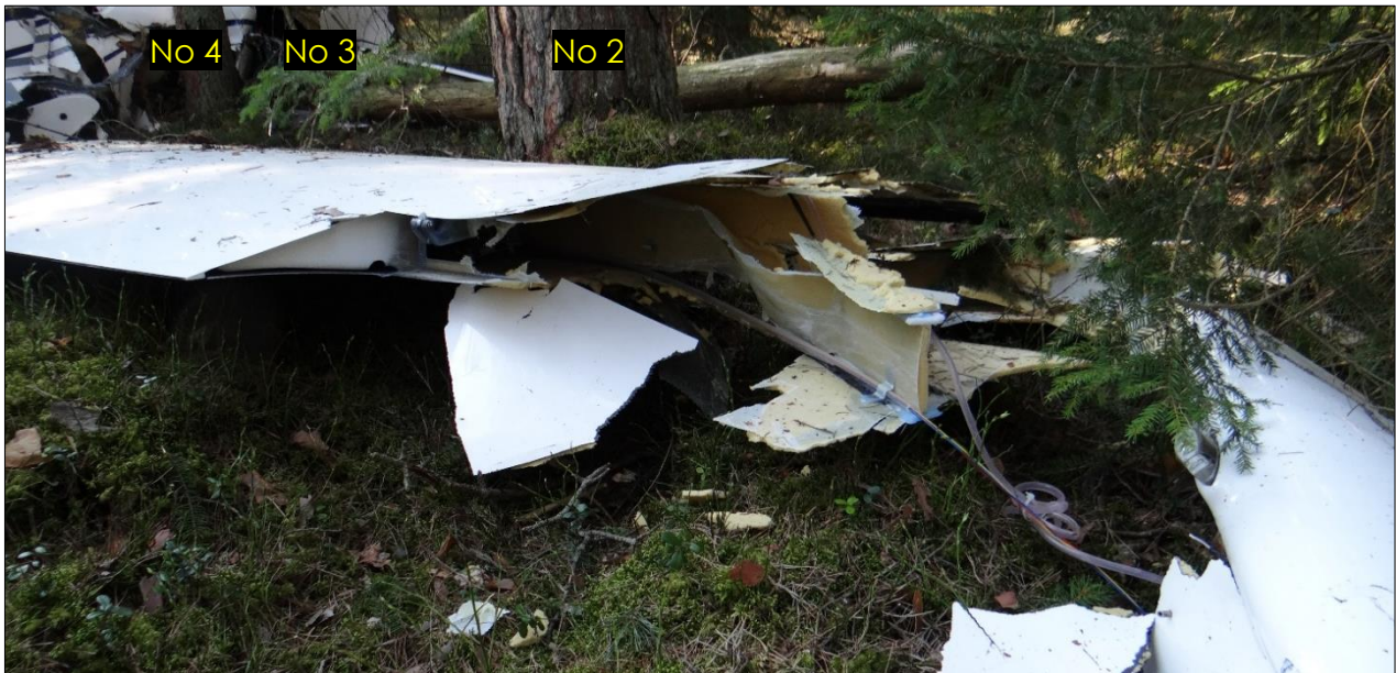
Fig. 12. Crashed tip of the right wing
