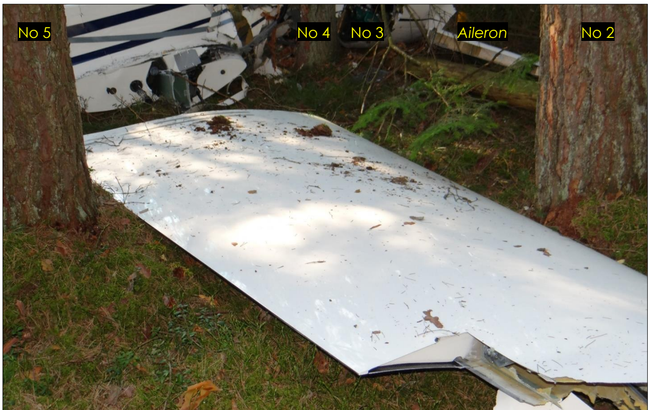
Fig. 11. Separated right wing between pines
