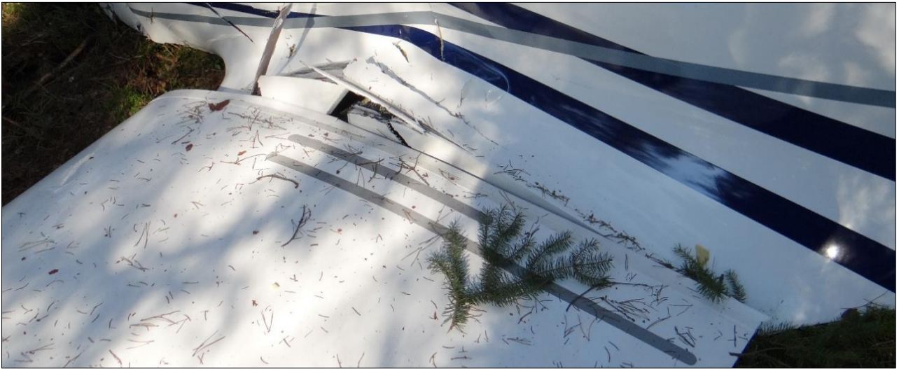
Fig. 10. Displaced left wing
