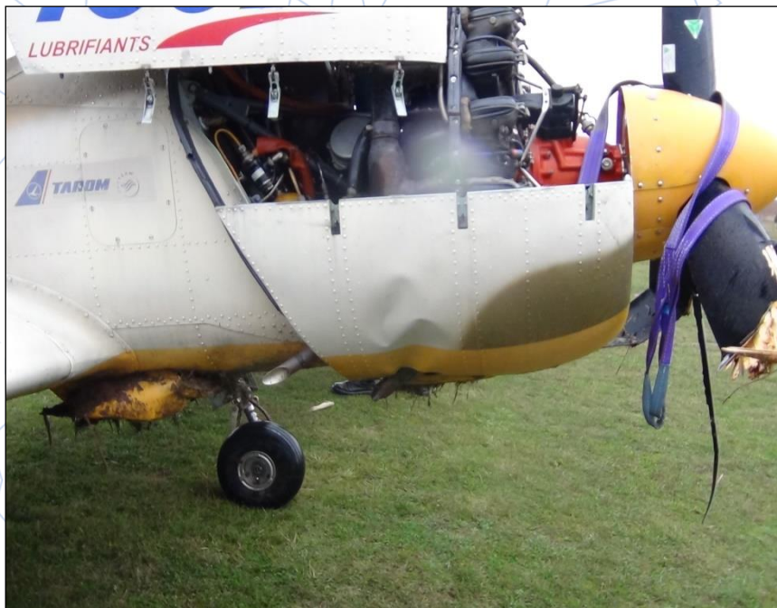
Fig. 4 Damaged engine lower cowl and propeller
