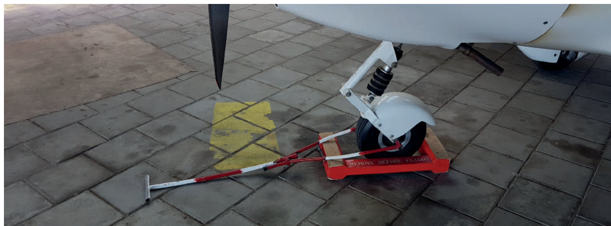
The tow bar attached to the nose wheel. (Photo: Police Aviation Division)
