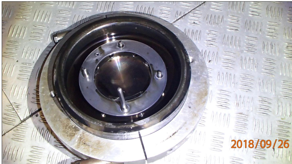
Fig. 8. Top steel part of the piston (bottom side) with broken holding bolts
