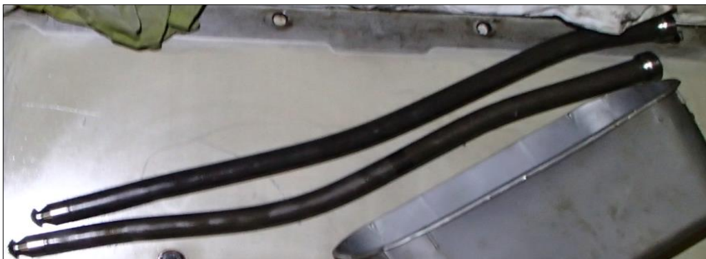
Fig. 5. Bended pushrods of cylinder No. 4
