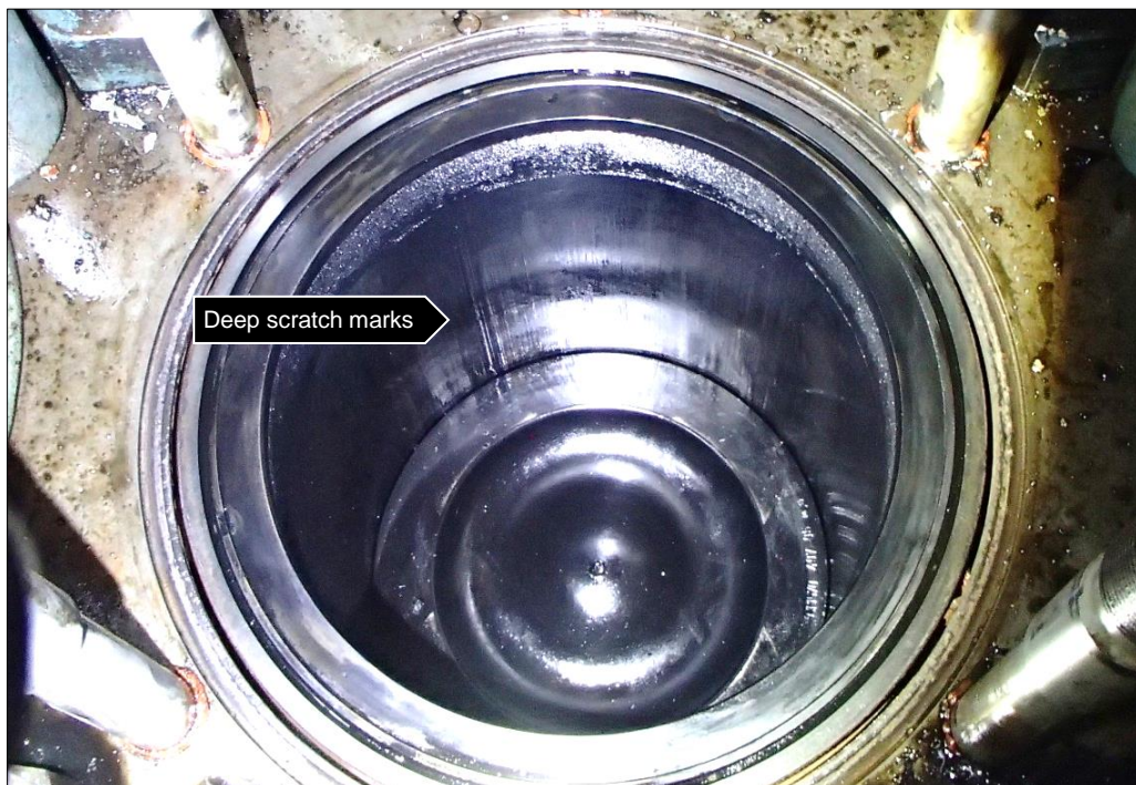
Fig. 9. Inner surface of cylinder No. 4 liner after the accident
