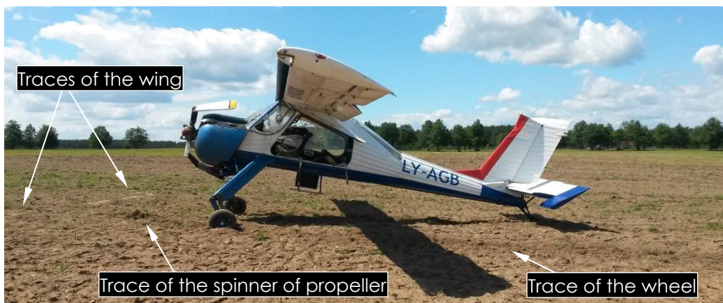
Fig. 3. Aircraft PZL-104 Wilga-35A at accident site after turning-over
