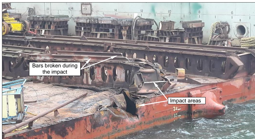
Fig. 10. Floating dock PD-408 after the accident
