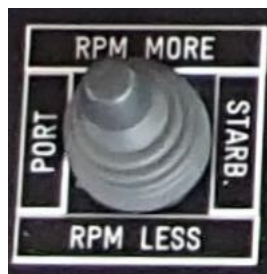
Fig. 8. Manual steering / power regulation joystick
