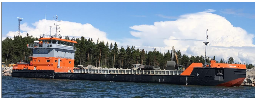
Fig. 2. Split hopper barge Boann (photo provided by the operator of seagoing ship)
