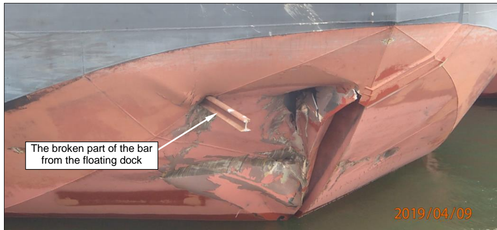
Fig. 9 Damages to the fore part of the Boann hull after the accident
