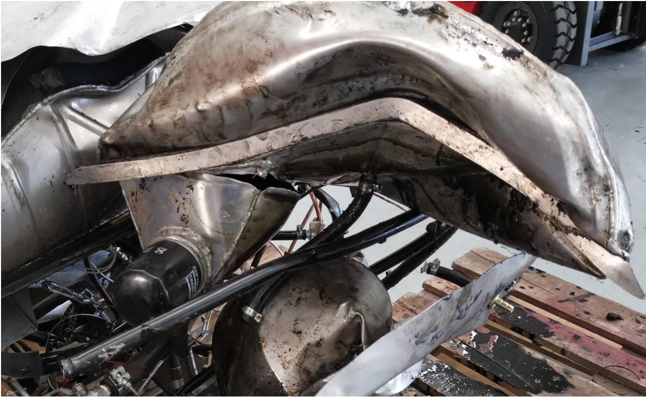
Picture 14: Damaged oil tank
