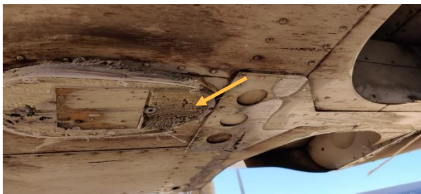
Photograph 8: Detached marker beacon receiver
