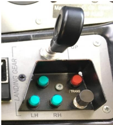
Photograph 20. Landing gear control panel
