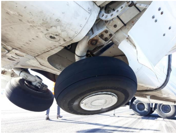
Photograph 21. Retracted main landing gear on the incident aircraft
