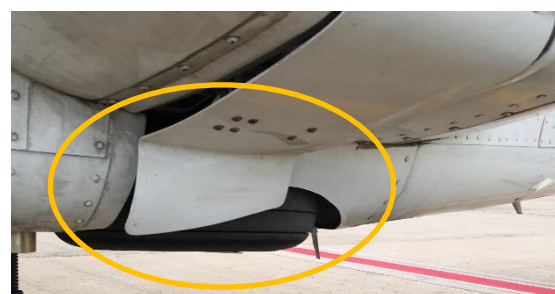
Photograph 18: Closed position of bent left MLG door
