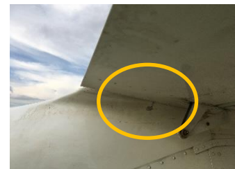
Photograph 12: Damage to right wing root
