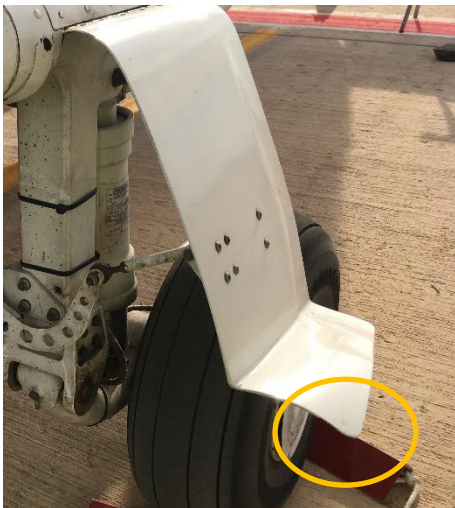
Photograph 15: Bent left MLG wheel well door
