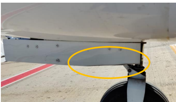
Photograph 17: Bent NLG door
