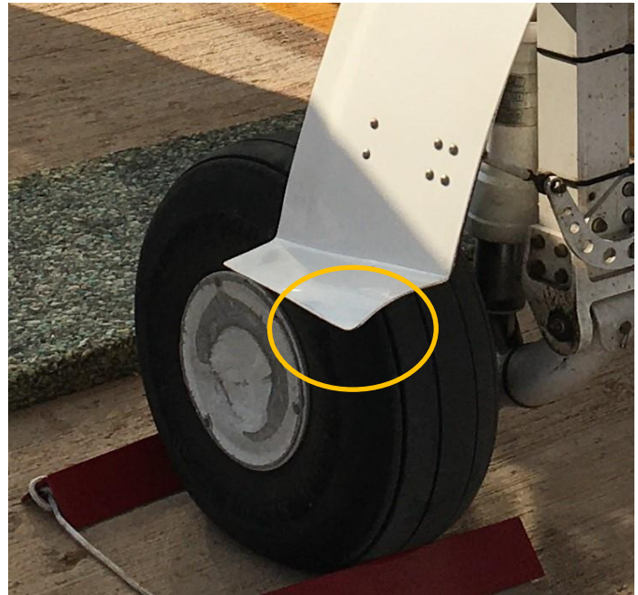
Photograph 16: Bent right MLG wheel well door
