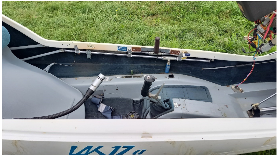
Figure 2: LAK17 cockpit In blue the speed brake control, in grey the flap control
