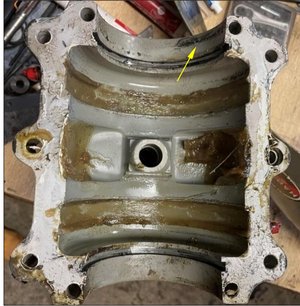
Fig. 7. Left propeller '-2BSF' blade impact mark on hub (yellow arrow)
