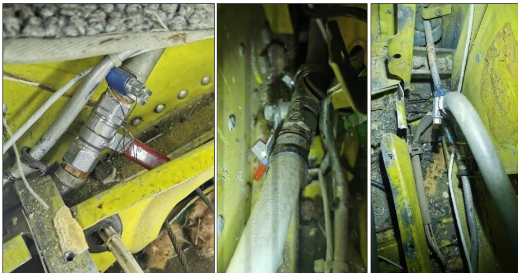
Fig. 10. Extraneous fuel system equipment
