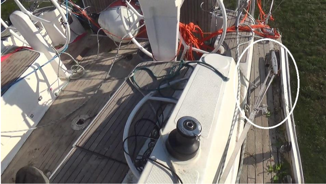
Photograph 13. Fastening of the jackstay on the stern (photo by M. Cesnauskis).
