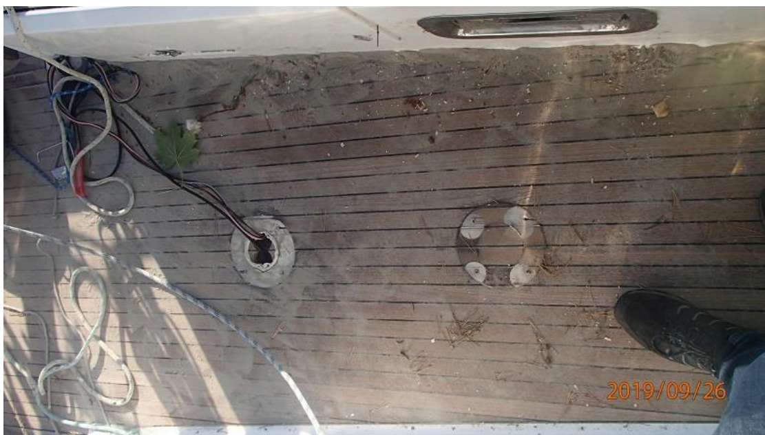
Photograph 12. Traces of screws securing the cockpit table (photo by M. Cesnauskis).
