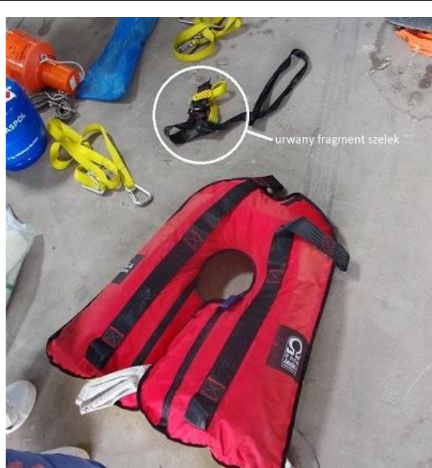
Photograph 9. Fragment of the harness torn off (photo by the SMAIC).
