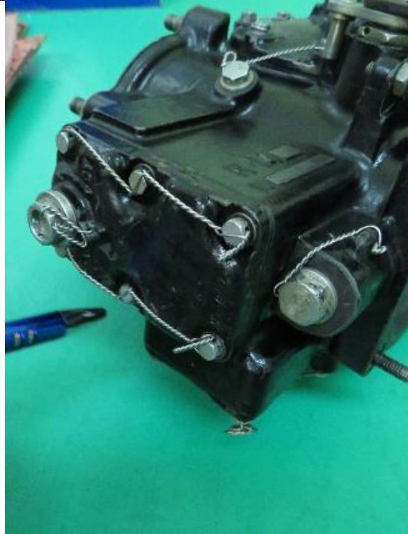
The seal on linkage lid (No. 173103) - missing Fig. 5.
