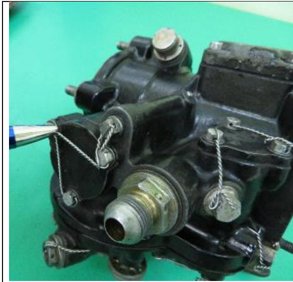
The seal on the accelerating pump lid (No. 173102) – missing; Fig. 7.
