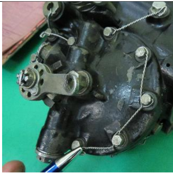
The seal on the diaphragm mechanism lid (No. 173 012-2) - missing Fig. 6.
