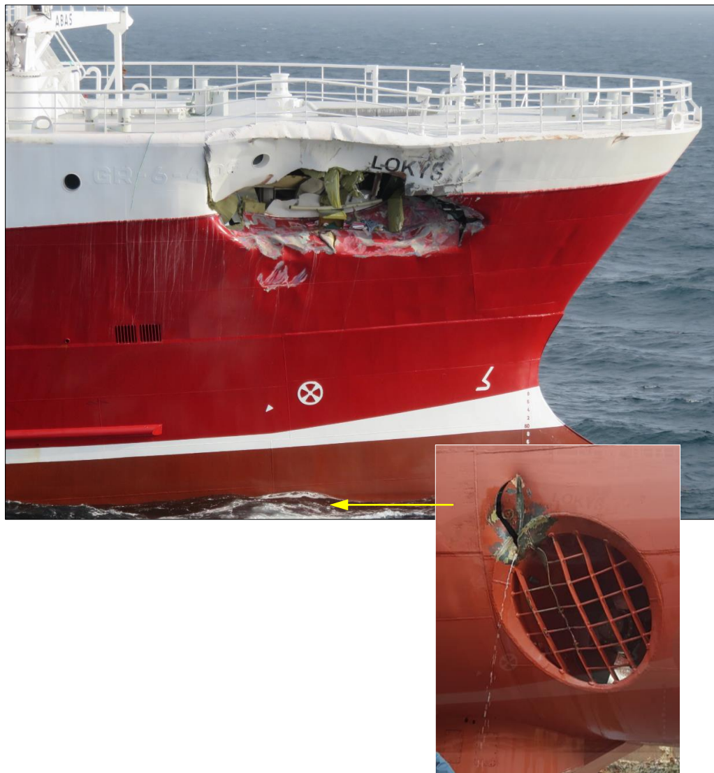
Fig. 6. Lokys starboard damages (photos provided by the operator of the ship)
