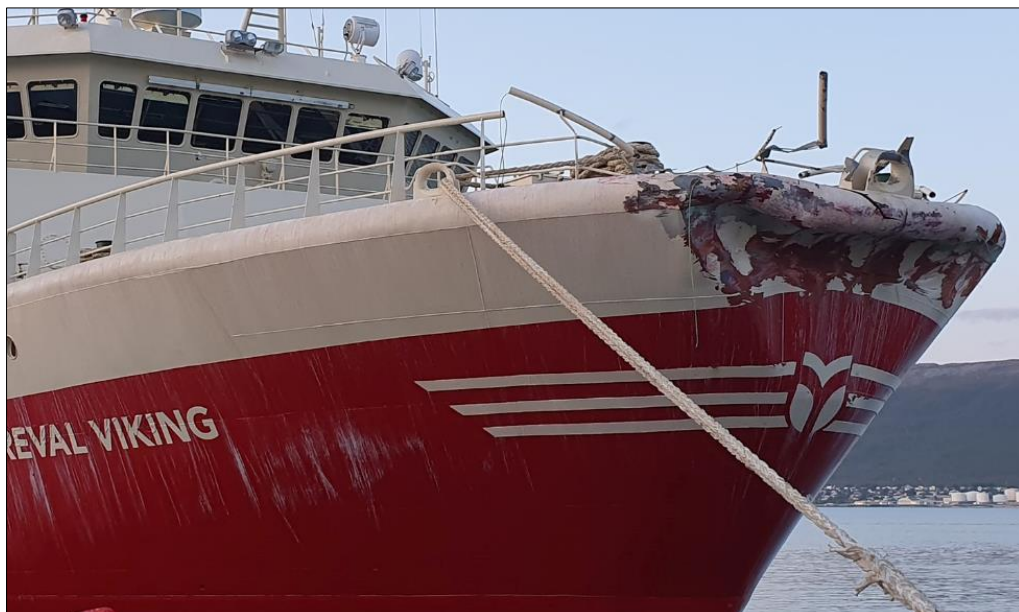
Fig. 5. Reval Viking bow damages (photo provided by the operator of the ship)
