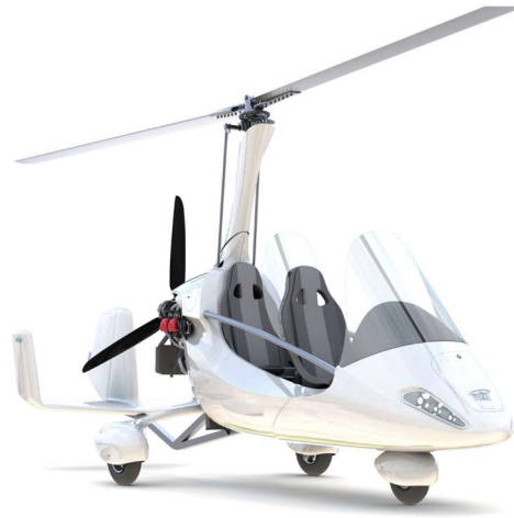
Fig. 7. MTOsport gyrocopter (Pilot Handbook for gyroplane MTOsport model 2017 915iS (issue date 14.08.2019, revision 1.1))
