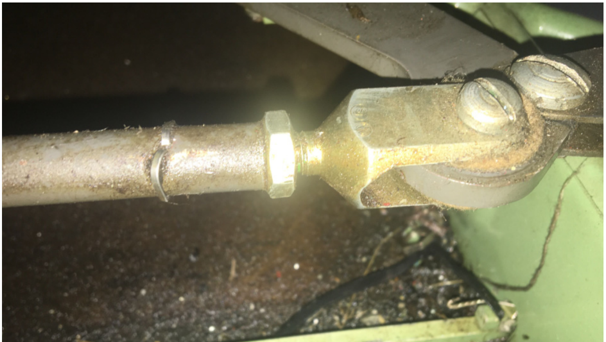
Photo 6: Example of the additional safety device (cotter-pin) at another Fw44J "Stieglitz" Source: Owner of a Fw44J "Stieglitz"
