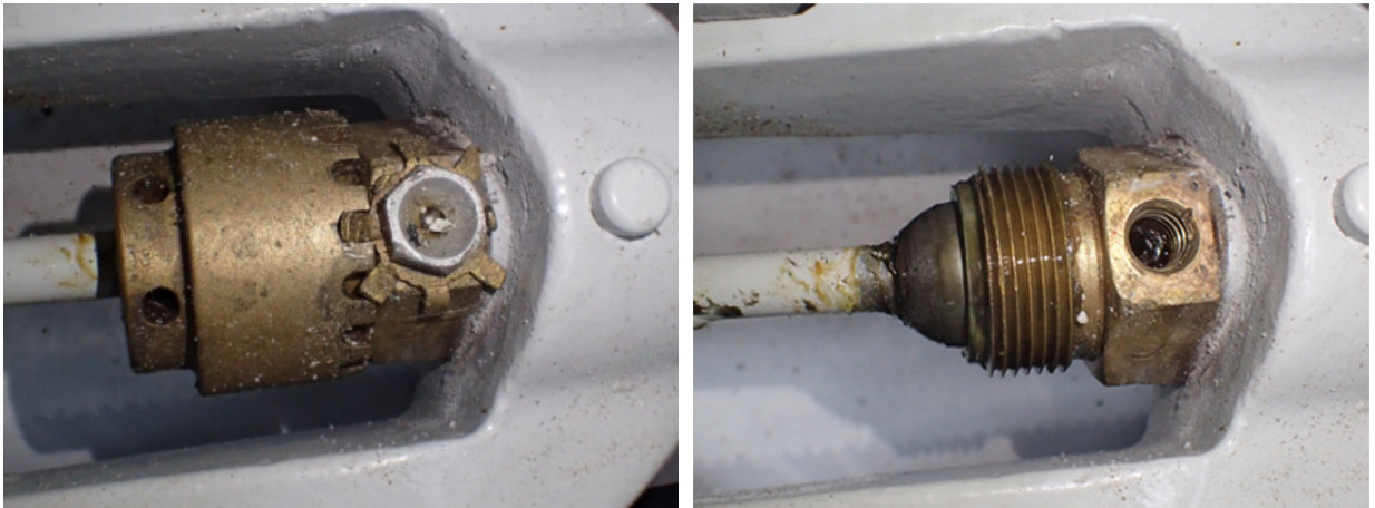
Photos 4 and 5: Front connection of the aft control rod with the control stick; with and without coupling nut Source: BFU
